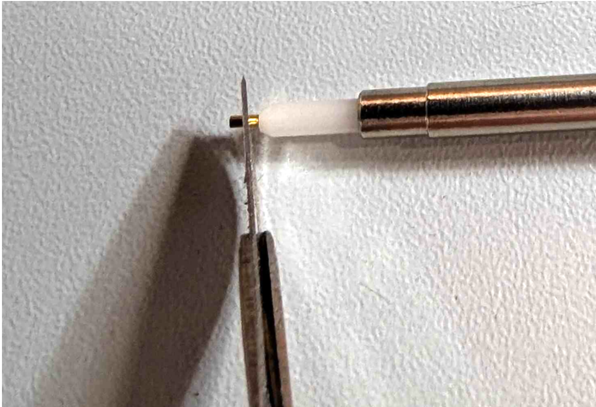
Fig 3. Cut the metal part, do NOT PUSH HARD, that will pinch the tube. Use a scalpel and cut/score a groove around the tube to create a break area so you can later break off the outermost piece to access the stuck needle.
